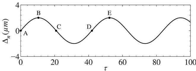
**Fig. 6.** Sinusoidal loading relation in the *normal* crack opening direction. The following portions of the loading history are delineated: loading (A-B), unloading (B-C), contact (C-D), and reloading (D-E).
