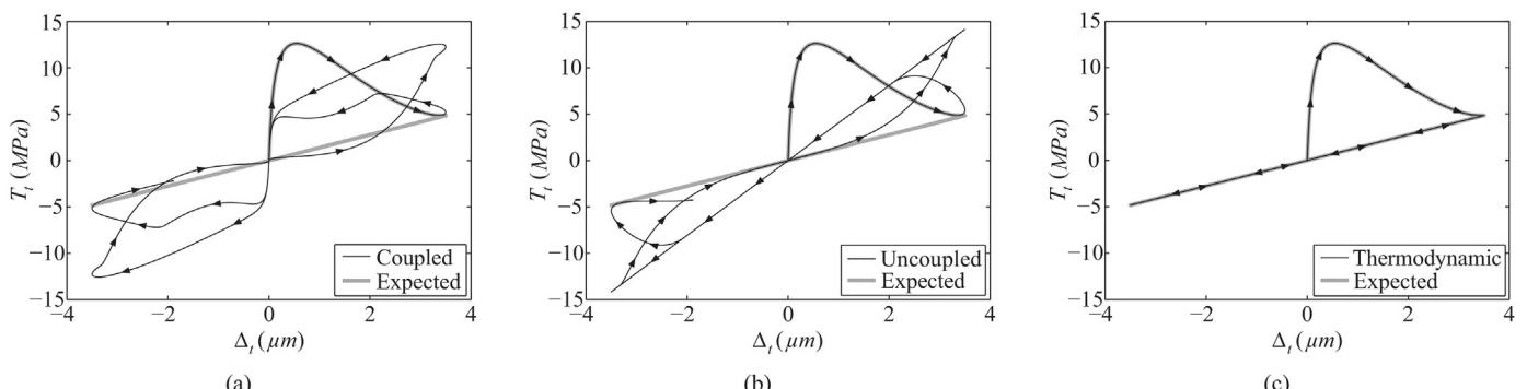
**Fig. 9.** Traction in the *tangential* direction during mixed-mode sinusoidal loading/unloading. Computed for the: (a) coupled, (b) uncoupled, and (c) thermodynamically consistent unloading/reloading relations.
