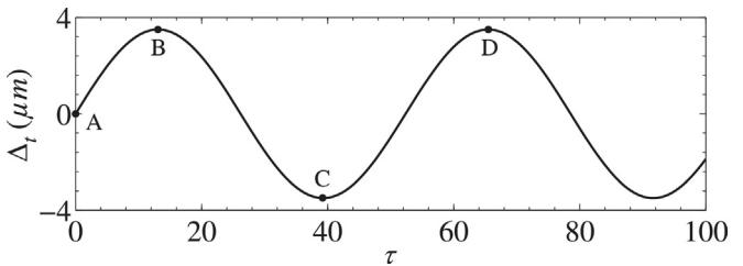
**Fig. 7.** Sinusoidal loading relation in the *tangential* crack opening direction. The following portions of the loading history are delineated: loading (A-B), unloading (B-C), and reloading (C-D).
