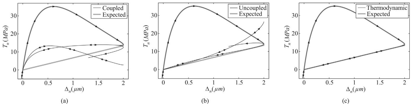
**Fig. 8.** Traction in the *normal* direction during mixed-mode sinusoidal loading/unloading. Computed for the: (a) coupled, (b) uncoupled, and (c) thermodynamically consistent unloading/reloading relations.
