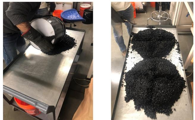
Fig. 3. Splitting the bucket of mixture as per AASHTO R47.
